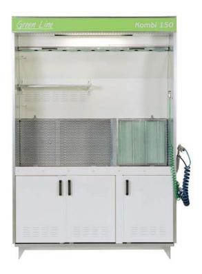
The Kombi 150 have three vital function within the same unit. Manual cleaning and inspection of spraying equipment is made in a rational manner to the cabinet's right side. It has a washing sink that holds 12 liters, the bottom of which has a perforated plate, so that for instance paint cups soaked in water does not come in contact with the sediment that occurs in all such washing vessels.
